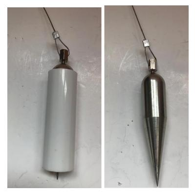
Thread the loop of the metal bob over one of the pronged ends and move it around the shaped clip; hold the clip so that the bob hangs from the indent in the bottom of the pronged clip.
