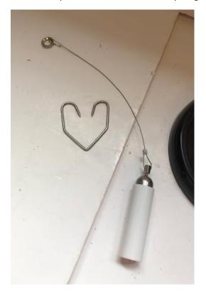
Remove the protective plastic sleeve from the metal bob – you may need to cut the plastic sleeve to loosen it and slip from the bob. Be careful to avoid touching the sharp tip of the metal bob.
